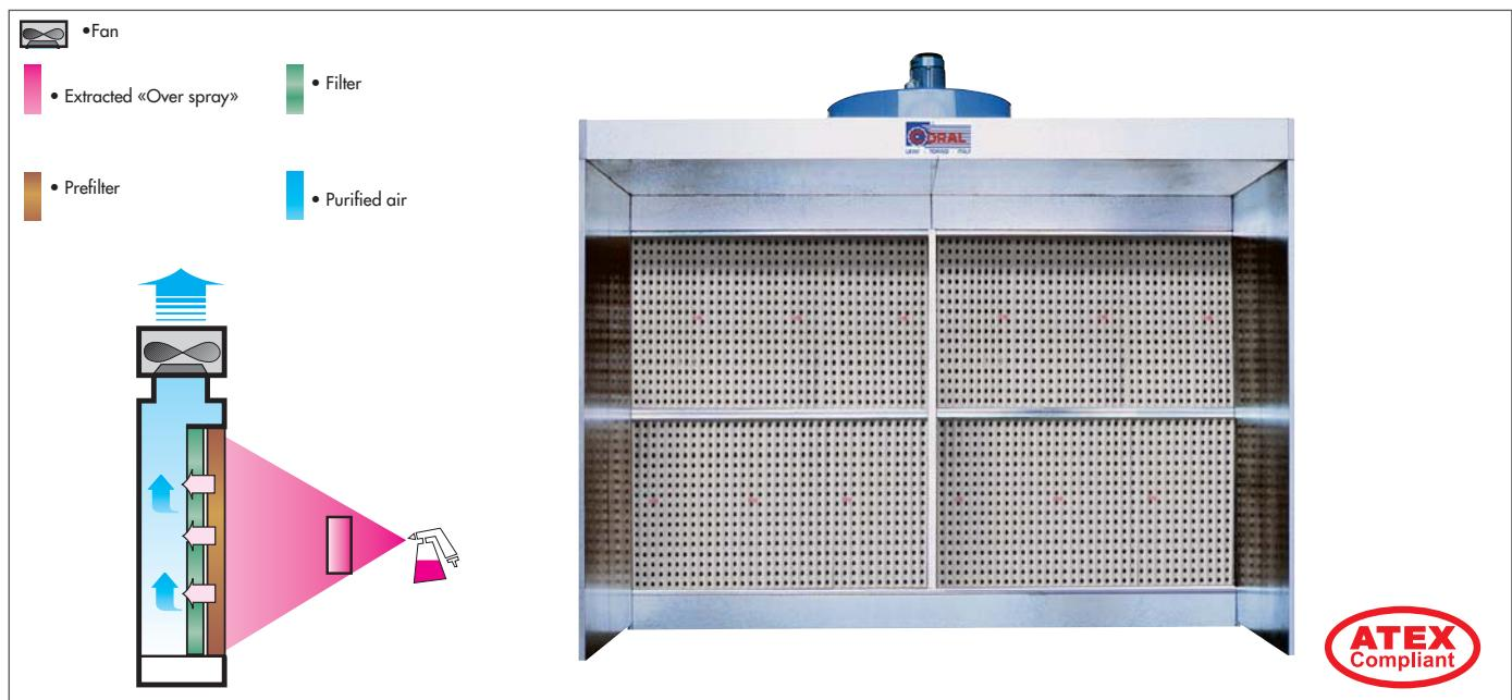
Valid for the same applications as the Tecnodry model. It is supplied with a double filter stage; thanks to its high-performance backward inclined sparkproof fan it uses less power and it is capable of optimizing extraction. Also available with extended walls and roof (version B), it is produced in two heights. Also available **ATEX COMPLIANT**.
